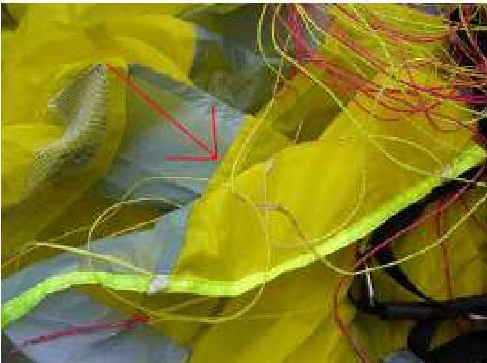
Figure 9: The ripping and burning effect on the wing surface.
