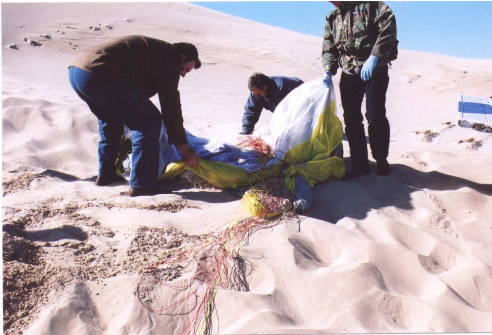
Figure 8: The condition of the wing when it was found.
