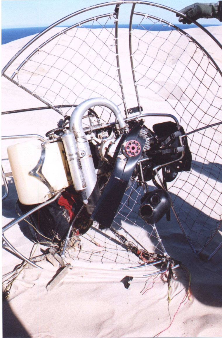
Figure 7: The damage sustained on impact with the ground.
