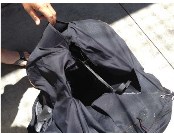
Fig. 3 Harness base tear
