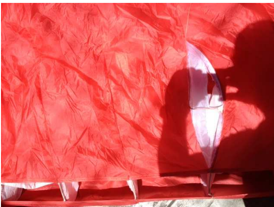
Fig. 1 Bottom skin cell wall burst
