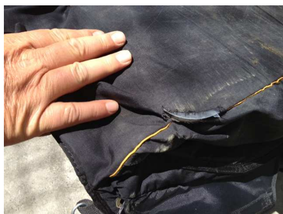
Fig.4 Harness frontal tear
