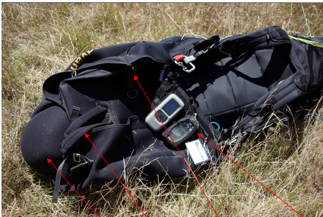
Harness showing Neoprene Skirt(1), leg straps(2), Skirt attachment (3) and Cockpit(4)
