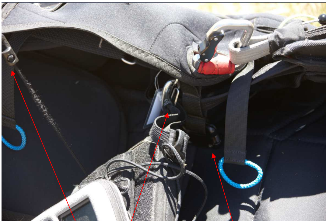
Close up view of the skirt (1) and cockpit(2) attachment indicating that they were done up. The one leg strap attachment is also visible(3)
