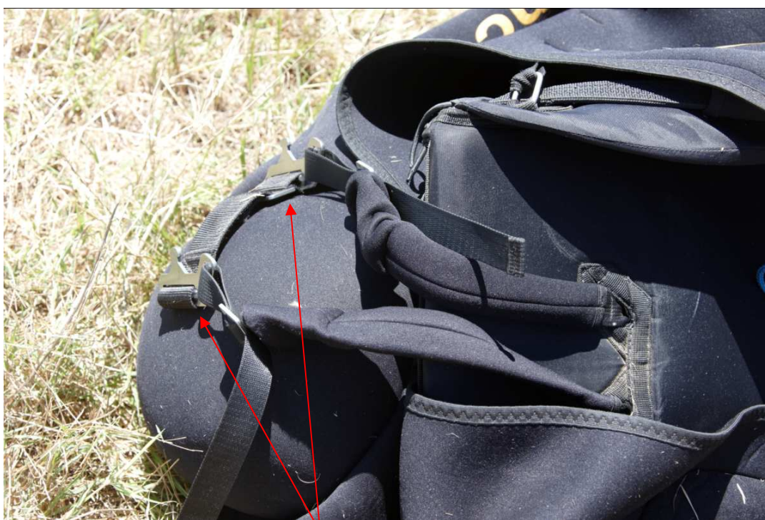
Leg strap buckles not done up
